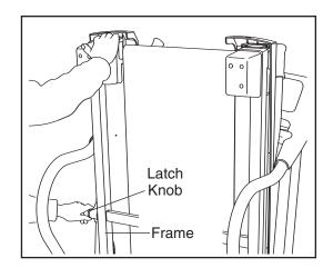
Hold the metal frame firmly with both hands, and lower it to the floor. CAUTION: To decrease the possibility of injury, do not lower the frame by gripping only the plastic foot rails.
